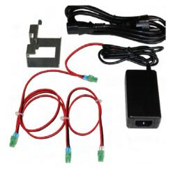
5VDC-4A power supply with a daisy-chain 4-plug output power cord. The cord length between succesive plugs is approximately 40cm, in order to be able to reach modules situated far away from each other in a cabinet. The power supply has a male IEC C14 mains input and comes with a IEC C13 to EURO (pin earth) cord. The power supply can easily be mounted in the cabinet by sliding the included mounting bracket into the suited slot at the bottom the abitana DIN-rail connectors.
